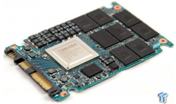
Figure 1: Example of SSD card with power loss protection function
